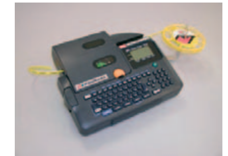
PRINTING ON PROFILE FROM A COMPACT DISC, MOUNTED ON THE REEL BRACKET.
