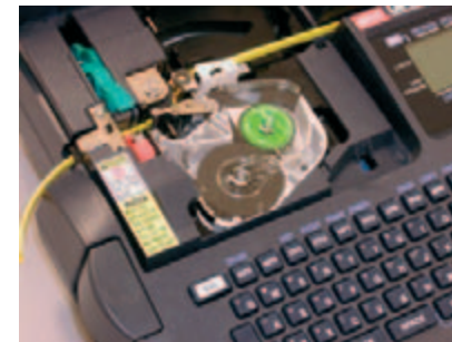
THE PICTURE SHOWS THE PROMARK RIBBON AND HOW THE PROFILE IS FED THROUGH THE MACHINE.
