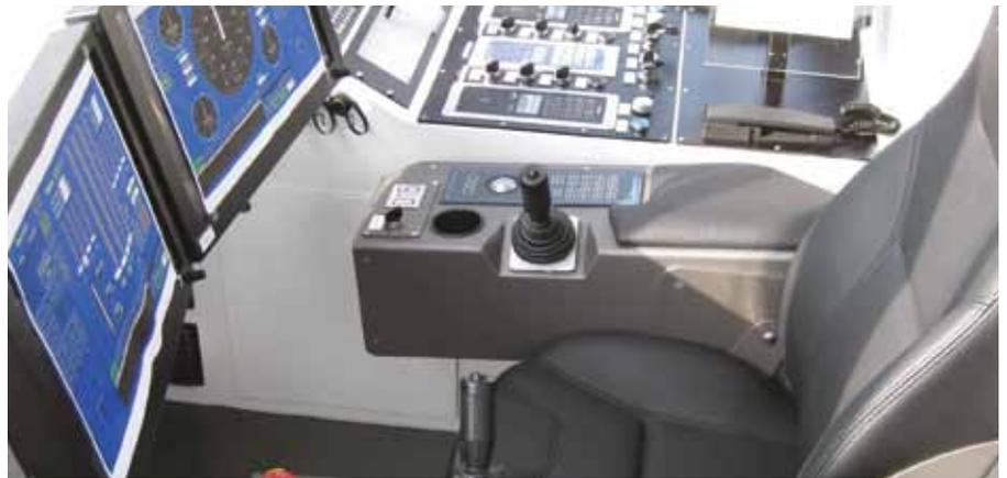
Modern lifting and moving machinery needs advanced control panels. Pushbuttons, joysticks and stop switches now share the same interface with data displays delivering real-time information. With an ever-increasing pool of technology, a new approach and understanding of HMI design and interaction is needed.
